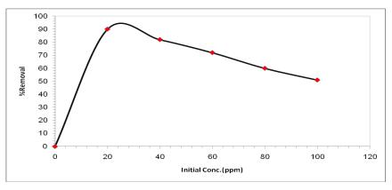
Fig (6) Effect of initial Conc. on the removal efficiency (Current density =20 mA/cm<sup>2</sup>, Initial pH=7, NaCl Concentration =1 g/l, Temperature =25°C, Time =120min)
