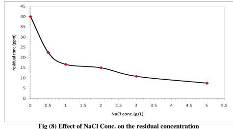
Fig (8) Effect of NaCl Conc. on the residual concentration (Current density =20 mA/cm<sup>2</sup>, Initial pH=7, Initial concentration=40 ppm ,Temperature =25°C, Time =120min)
