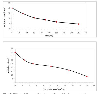
**Fig (5) Effect of Current Density on the residual concentration** (Initial pH=7, **Initial** concentration=40 ppm, NaCl Concentration =1 g/l, **Temperature** =25°C, Time =120min)
