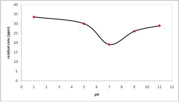
**Fig. (7) Effect of pH on the residual concentration** (Current density =20 mA/cm<sup>2</sup>, Initial concentration=40 ppm NaCl Concentration =1 g/l, Temperature =25°C,Time =120min.)
